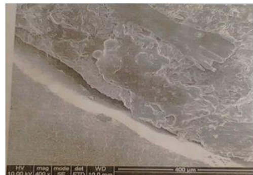
Figure: 2b SEM of Polyurethane with 20% hydroxyapatite (HA) after push out test
