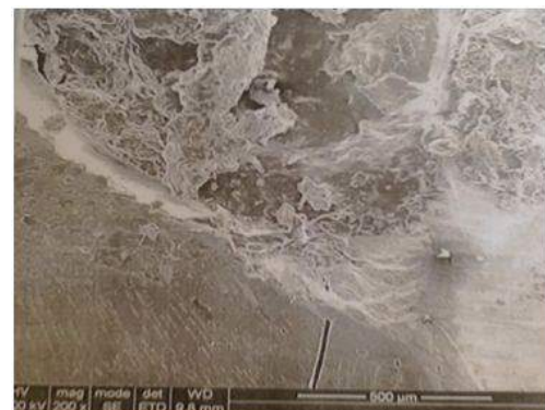
Figure: 2b SEM of Polyurethane with 20% hydroxyapatite (HA) after push out test
