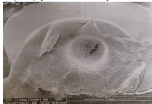
Figure: 2a SEM Of Polyurethane with 10 hydroxyapatite (HA) after push out test
